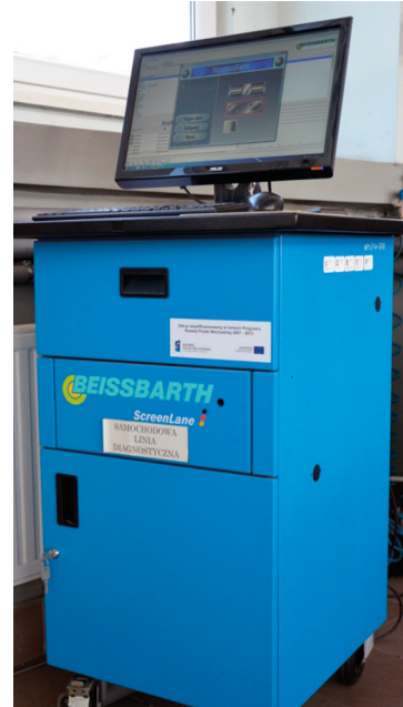
Figure 2. Control system of the Bosch Beissbarth SA 640 test stand
