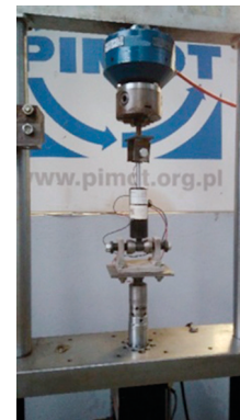
Figure 2. Testing the damper in the test station
